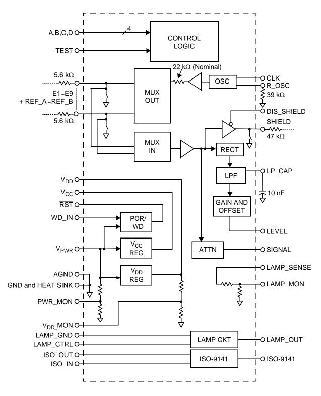
Figure 1. 33794 Internal Block Diagram
